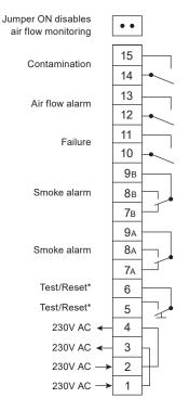
The relay outputs are shown in power off/alarm condition.
